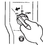
3. Turn the fuel valve to the “OFF” position.
