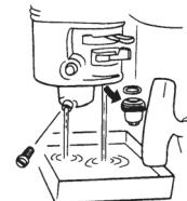
3. Remove the drain plug and drain the oil.
