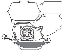
2. If the oil level is low. Fill the oil to the upper level.
