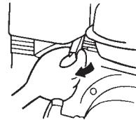
3. Turn the choke lever to the close position.
