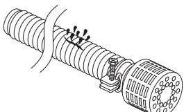
Is the hose band installed securely?
