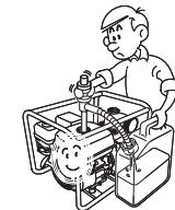
2. Drain the fuel from the carburetor.
