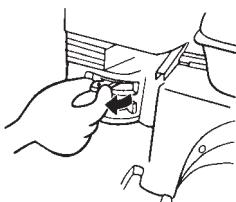
4. Turn the engine switch to the "ON" position.
